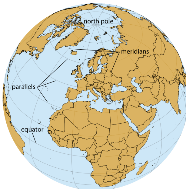
Figure 15-1. Orthographic projection of the world, showing Europe and Northern Africa as they would be visible from space. The lines emanating from the north pole and running south are called meridians, and the lines running orthogonal to the meridians are called parallels. All meridians have the same length, but parallels become shorter the closer we are to either pole.
