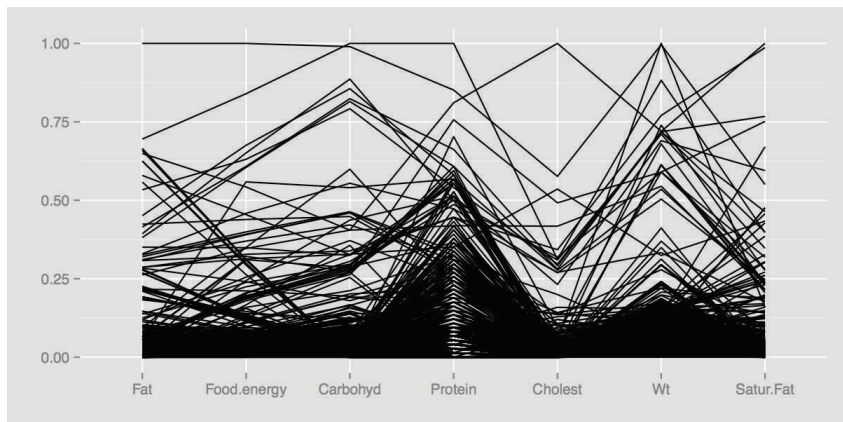
FIGURE 6.1: A parallel coordinate plot of the seven variables in the food dataset from the MMST package. There are outliers and all the distributions look skewed to the right, because most of the lines are packed into the foot of the plot. Setting scale="uniminmax" means that each variable is scaled individually from its minimum to its maximum.
