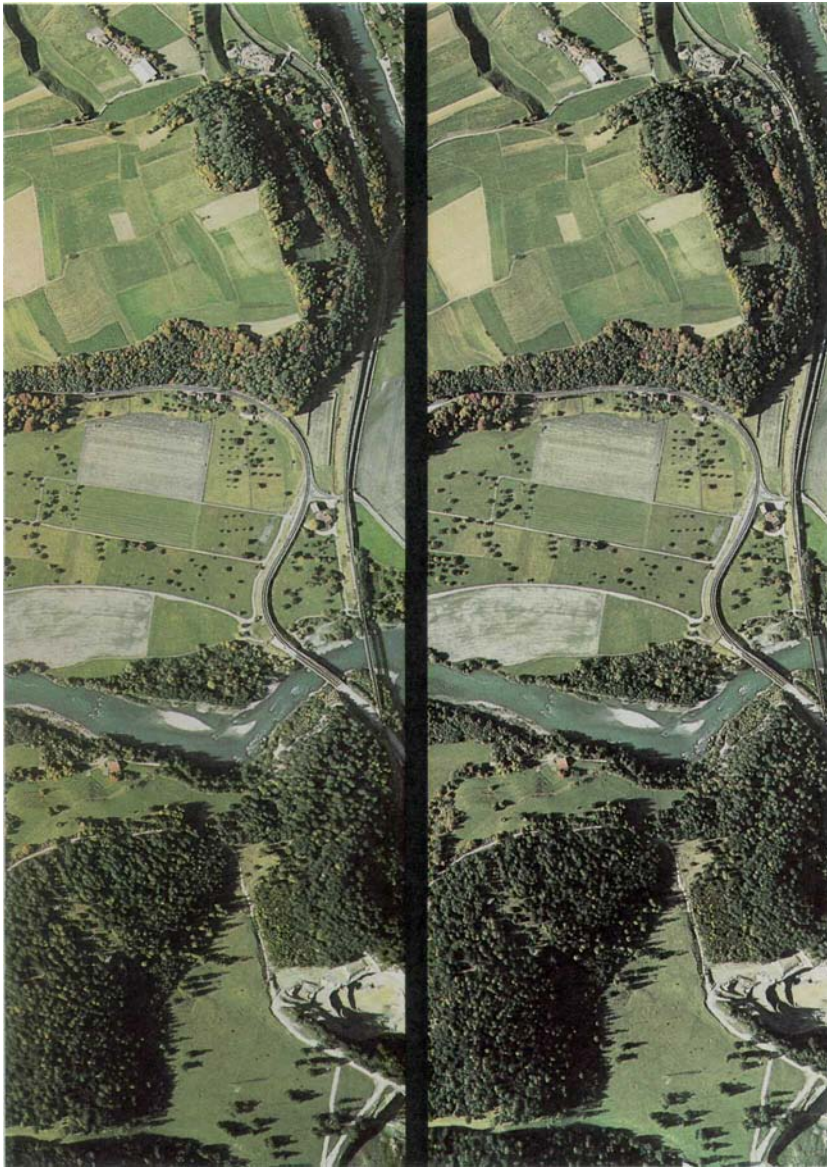
Color stereopair of Bonaduz, Canton of Grisons, Switzerland, October, 1975, photographs taken with Wild Leitz aerial camera RCIO. Scale about 1:11,000.
