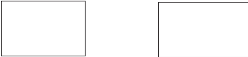
Figure 1.6 Comparison of a rectangle 50% wider than tall (on the left) with a rectangle with dimensions defined by the Golden Section (on the right)
