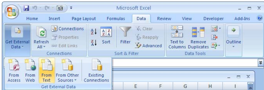
Fig. 3.27 To read data directly into Excel, we can use the Excel Data ► Get External Data ► menu. We show one more step here, the From Text item. Once the dataset is in Excel, we can access it using the techniques illustrated in Sections 3.2–3.5.
