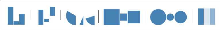
Figure 5-5. Difficulty in comparison increases roughly from left to right: comparing length with a shared baseline and with different baselines, comparing angles, comparing square areas or circular areas, and comparing color. Each of these shows three values in the proportion 5:1:3.
